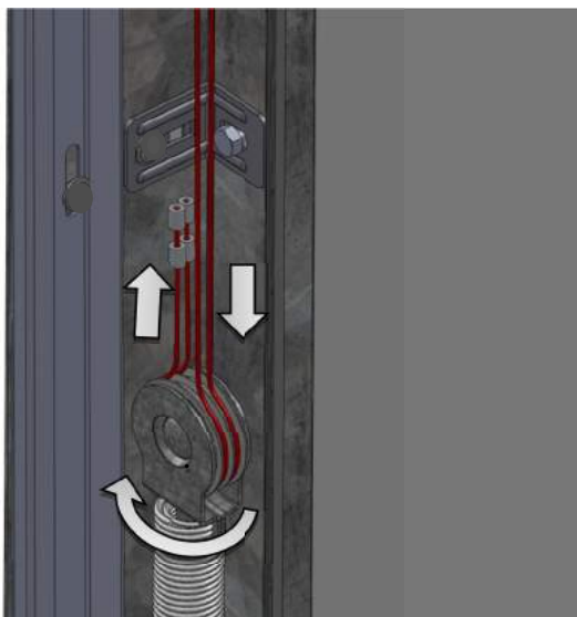
Figure 36: cable installation – step 2
